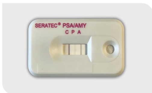
Figure 1: Test Card Layout PSA (P), \alpha -amylase (A) and control (C)
