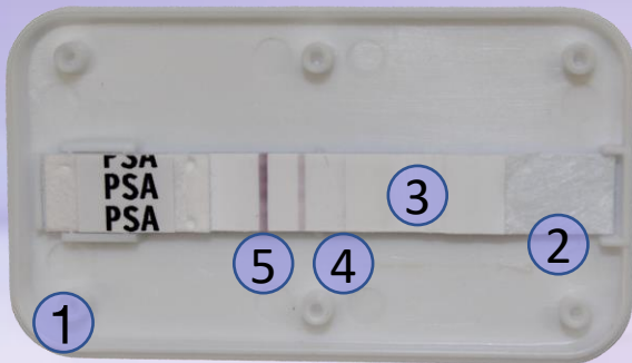
Fig. 1. SERATEC® test strip inside an open test card after reaction. An extract was placed on the sample pad and flowed along the test membrane. Both test result line and control line are clearly visible.
