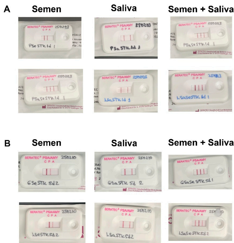
Figure 6. PSA and \alpha -amylase detection alone and in combination just after deposition, showing plastic (top) and leaves (bottom) (A) or after 5 days post-deposition, showing glass (top) and leaves (bottom) (B).
