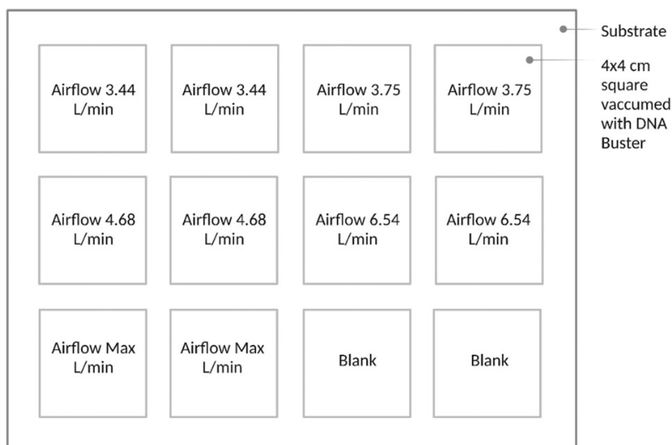
Fig. 3. Exemplary sampling allocation on a piece of cloth for different recovery methods with 4 cm × 4 cm sized sampling areas. Sampling areas were separately randomized across the cloths to minimize any bias related to the handling of the item. Created with BioRender.com [28].
