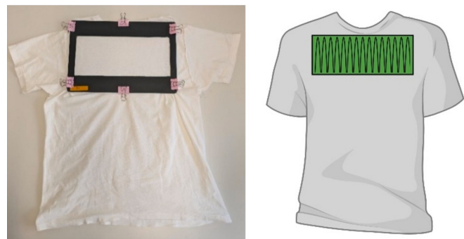
Fig. 1. Stencil fixation and vacuum direction. Left: Stencil that is secured with six clips in the middle of the T-shirt and touching the sewing line of the collar at the top. Right: Sampling area (green) that was vacuumed vertically from top to bottom (created with BioRender.com ). (For interpretation of the references to colour in this figure legend, the reader is referred to the web version of this article.)
