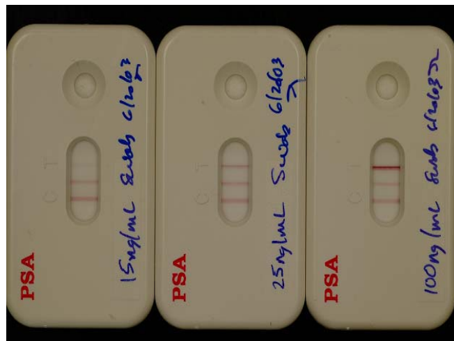
Figure 3. Results of the extraction of 15, 25 and 100 ng PSA/mL samples from cotton-tipped swabs. A band equal in intensity to the 4 ng/mL internal standard is visible in the 25 ng/mL sample.
