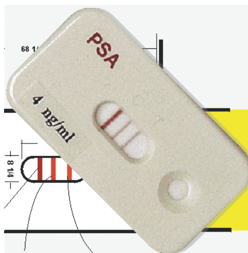
Figure 2. A Positive Reaction for PSA with the Seratec Kit (From Seratec's website, www.seratec.com .)
