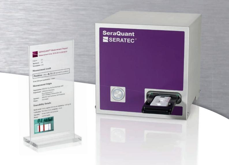
The SeraQuant is an instrument for the computer-based, quantitative analysis of the SERATEC® test kits and the automatic, consistent result documentation.
